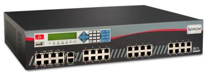
E1/T1 port. The XE2000 supports up to 160 PSTN / Analog phones ports with external Astribank units, up to 200 users and up to 85 concurrent calls.
